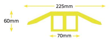
T-Matting is a new and unique innovation, designed specifically for 'Narrow' and 'Micro' trenching applications, exclusive to CID and has been developed in conjunction with contractors, local authorities and network providers around the UK.
