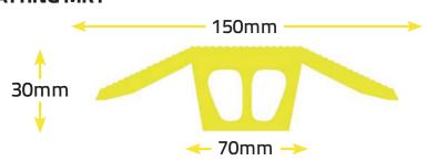
T-Matting is a new and unique innovation, designed specifically for 'Narrow' and 'Micro' trenching applications, exclusive to CID and has been developed in conjunction with contractors, local authorities and network providers around the UK.
