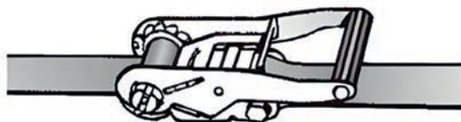
Lower the lock in the handle to the flat position.
