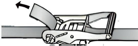
To thread, pull webbing through the slot in the centre rotating spool of the closed ratchet. Remove the slack.
